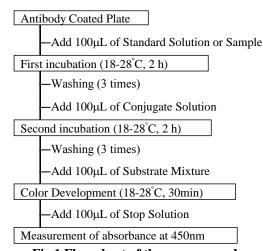
Fig.1 Flow chart of the assay procedure
