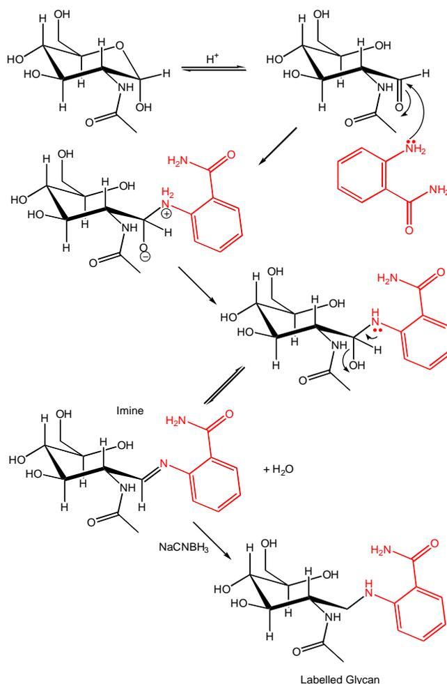
Figure 1: Labeling of a glycan with 2-aminobenzamide acid (2-AB) by reductive amination.
