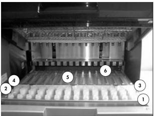
Figure 5. Worktable of an EZ1 Advanced XL instrument.
