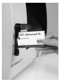
Figure 2. Ease of protocol setup using EZ1 Advanced XL Cards. Inserting an EZ1 Card, containing a protocol, into the EZ1 Advanced XL instrument.
