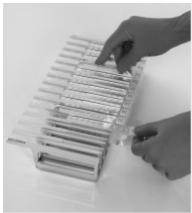
Figure 4. Ease of instrument setup using reagent cartridges. A A sealed, prefilled reagent cartridge of the EZ1 ccfDNA Mini or Midi Kit. B Loading reagent cartridges into the cartridge rack. The cartridge rack itself is labeled with an arrow to indicate the direction in which reagent cartridges must be loaded.
