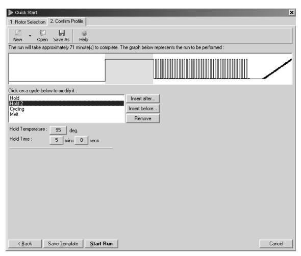
**Figure 5. PCR initial activation step.** After reverse transcription is completed, PCR can be carried out. PCR requires an initial incubation at 95°C for 5 min.
