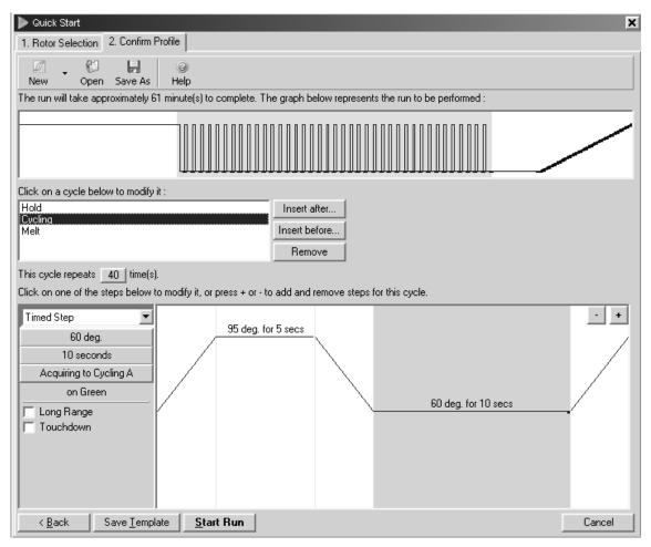
**Figure 2. Two-step cycling.** PCR requires 35–40 cycles. Each cycle is comprised of 2 steps: 95°C for 5 s (denaturation step) and 60°C for 10 s (annealing/extension step).
