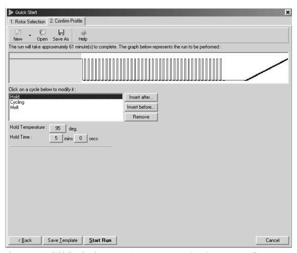
**Figure 1. PCR initial activation step.** PCR requires an initial incubation at 95°C for 5 min to activate HotStarTaq *Plus* DNA Polymerase.
