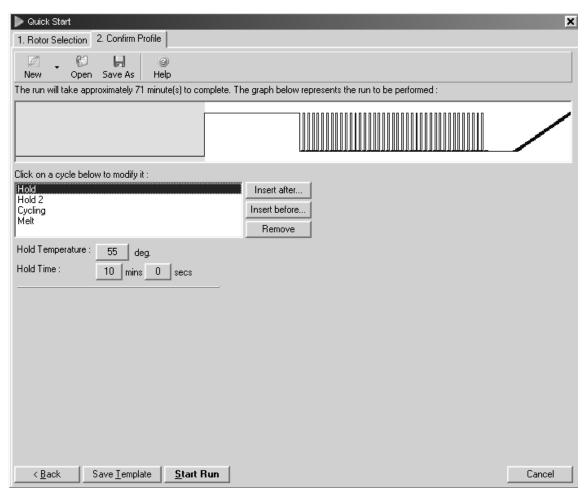
**Figure 4. Reverse transcription.** Before starting PCR, reverse transcription must be carried out. Reactions are incubated at 55°C for 10 min.
