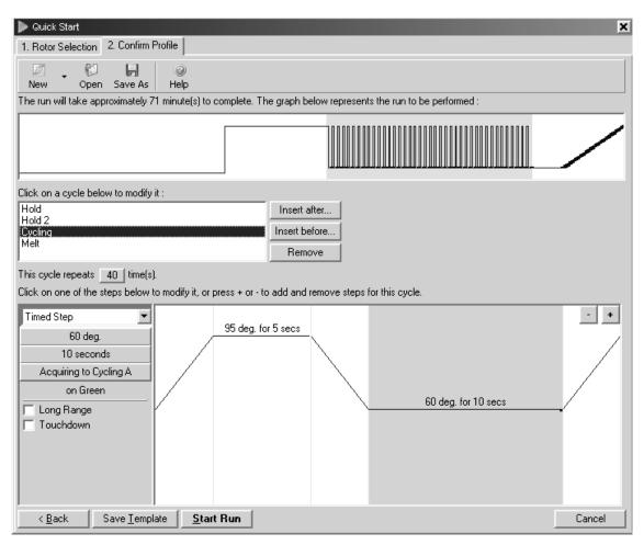
**Figure 6. Two-step cycling.** PCR requires 35–40 cycles. Each cycle is comprised of 2 steps: 95°C for 5 s (denaturation step) and 60°C for 10 s (annealing/extension step).
