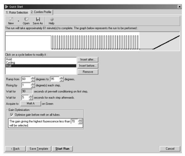
**Figure 3. Melting curve analysis.** After PCR is completed, melting curve analysis can be performed to check the specificity of the reaction.
