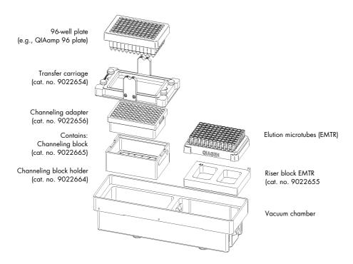
Figure 1. Assembling the vacuum chamber.
