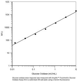
Glucose oxidase dose response was measured with Amplite™ Fluorimetric Glucose Oxidase Assay Kit in a solid black 96-well plate using a Gemini fluorescence microplate reader (Molecular Devices).
