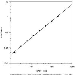
NADH dose response was measured with Amplite™ Colorimetric NADH Assay Kit in a 95-well white/clear bottom plate using a SpectraMax microplate reader (Molecular devices).
